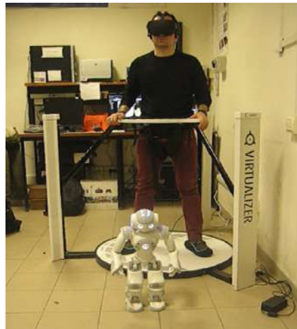
Figure 6.5. A photo taken from a test with a real robot: at the start of the simulation it is advisable not to move the head in order to avoid any malfunctioning of robot's one
